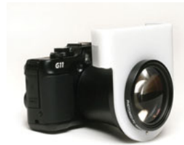
Figure 6. PhotoMed equipped Canon Powershot G11 point-and-shoot system.
